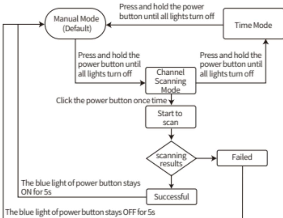
Time Mode: Use the programmable schedule to control the ON/OFF state of the Smart Plug, its own power button cannot control its ON/OFF.
